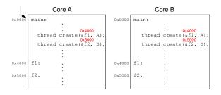
Figure 8: Identical Program Code On Each Node
