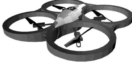
Figure 3: 3D model of the Parrot AR.Drone. This is a model optimized for simulation, based on the highly detailed model provided by Parrot SA.
