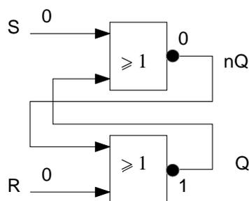
Assume that the top NOR-gate delays all changes by 2 ns, the NOR-gate at the bottom delays all changes by 3 ns. Assume that for  $t < 0$ , signal values are as indicated in the timing diagram below. At  $t = 0$ , R is assumed to change to '1'. Depict the waveforms at the outputs nQ and Q of the two gates, as computed by discrete event simulation!
