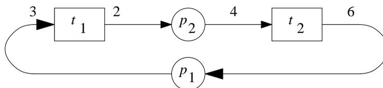
Which combinations of markings of  $p_1$  and  $p_2$  are feasible? Create a graph with  $(M(p_1), M(p_2))$  as nodes and indicate possible transitions. Start with a node  $(9,0)$ .
