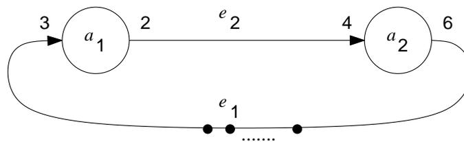
Suppose that SDF actors execute in 1 unit of time. Generate a possible execution schedule, assuming a single execution unit (no parallel execution) and an initial set of 6 tokens for edge  $e_1$ :
