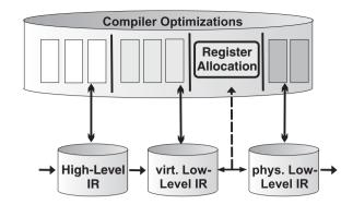
Figure 2. Internal code representation within the WCC compiler.
