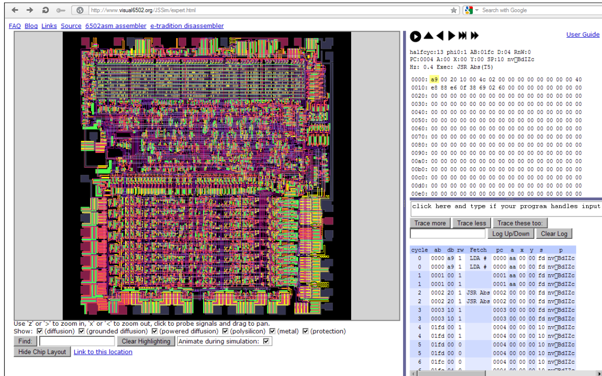
Figure 2.2: Screenshot of the interactive 6502 simulator from the Visual6502 project
