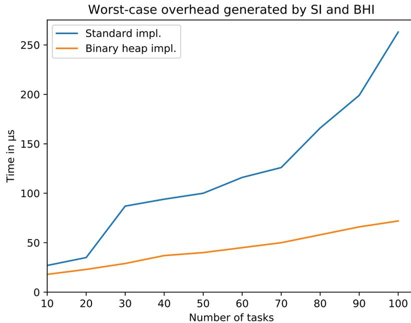
**Figure 3.4:** A comparison of generated overhead by the standard implementation(SI) and the binary heap implementation(BHI)
