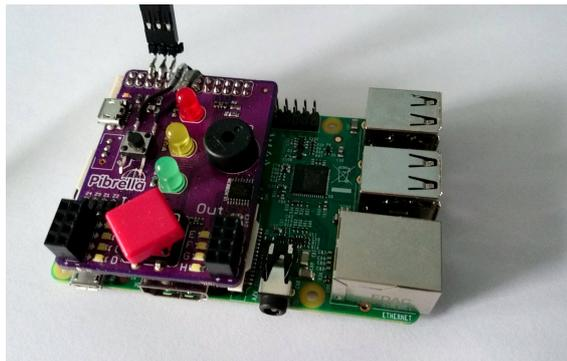
**Figure 3.6:** The Raspberry Pi B+ with attached Pibrella Board
