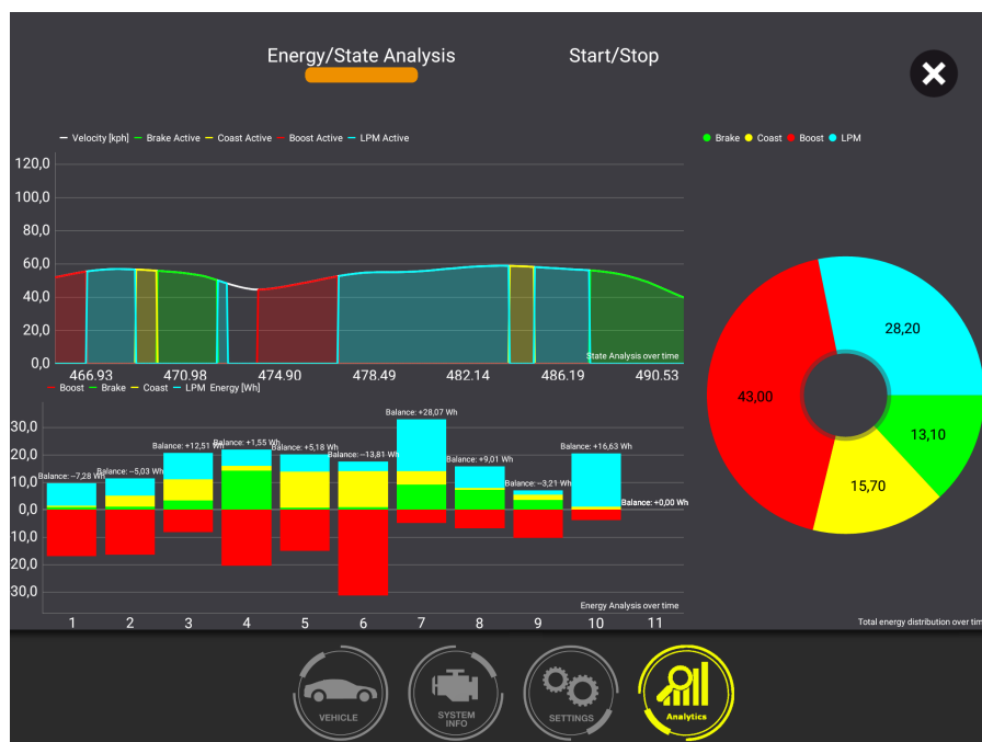
Figure 6.11: Representation of the energy behavior of all states and a distribution over time.
