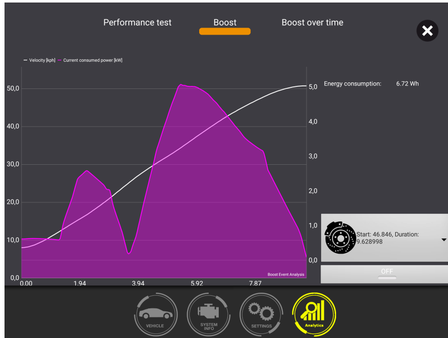
Figure 6.9: Representation of the energy behavior of a single boost event over time.
