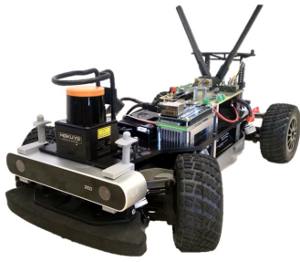
Fig. 1: The remote-controlled car based on the Traxxas Fiesta ST platform after modifications and augmentation of sensors (without the chassis).
