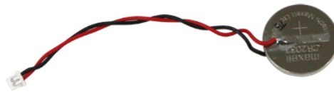
Figure 4.9: Backup Battery for the Real Time Clock for Odroid XU 4 [5]
