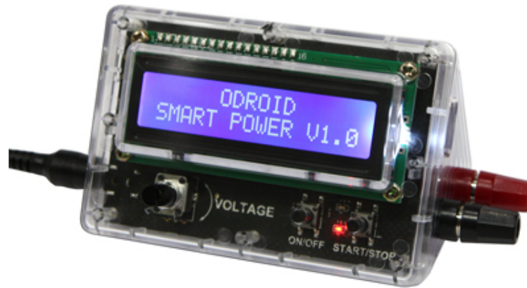
Figure 4.12: Smart Power module for measurements with Odroids [5]
