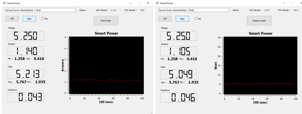
Figure 6.3: Graphical illustration for unconnected keyboard with optimized parameter on the Odroid. In the left figure the electric current intensity and in the right picture the power consumption while running the software is illustrated.
