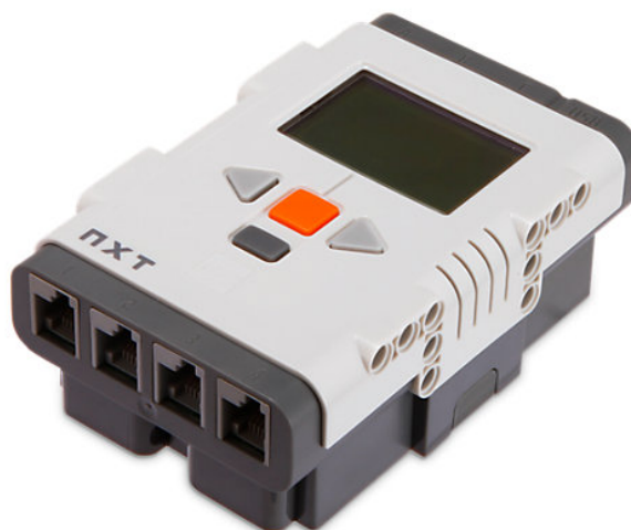
Figure 4.1: The Lego Minstorms NXT brick. All pictures of photos of the robot are from shop.lego.com
