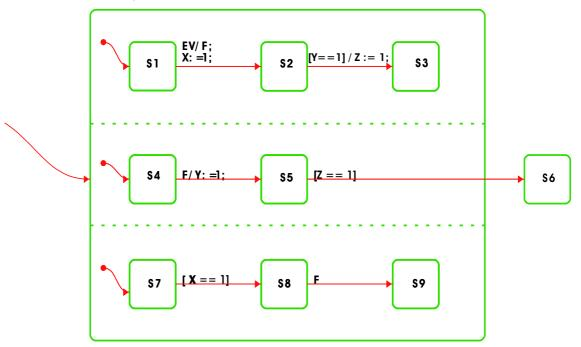
Describe all events and actions within this state chart given that event EV occurs in the first configuration (i.e. when states S1, S4 and S7 are active). Determine the particular configurations for each step and fill out the table (see next page). Explain why the transition S8  $\rightarrow$  S9 can never switch.
