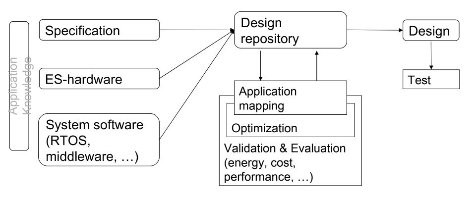
Generic loop: tool chains differ in the number and type of iterations
