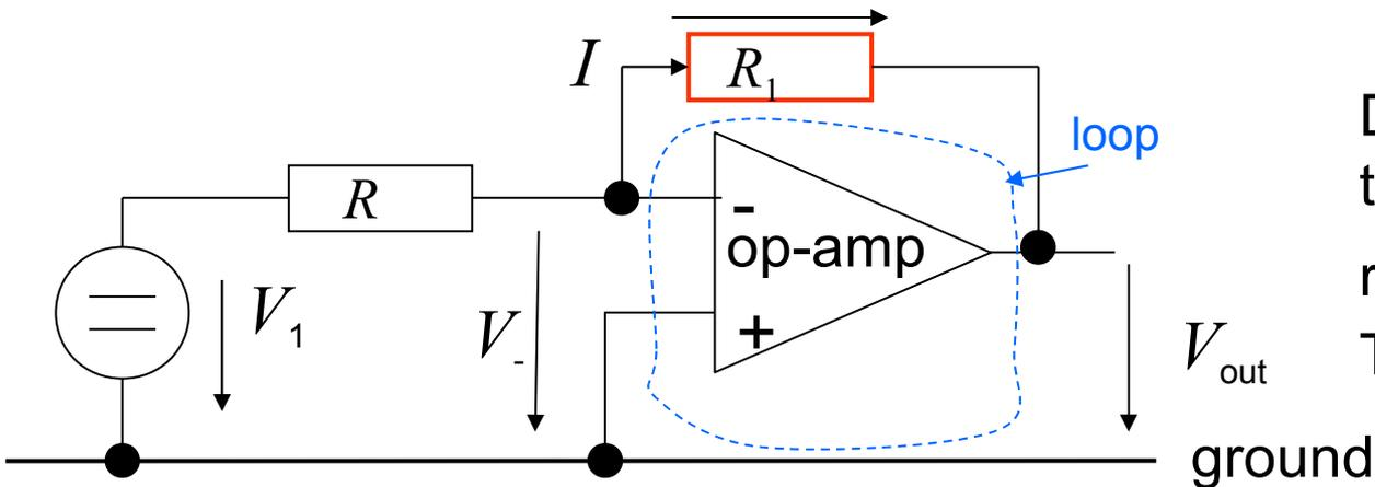
Due to the feedback to the *inverted* input,  $R_1$  reduces voltage  $V_-$ . To which level?
