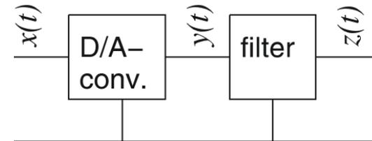
Filter removes high frequencies present the step function  $y(t)$
