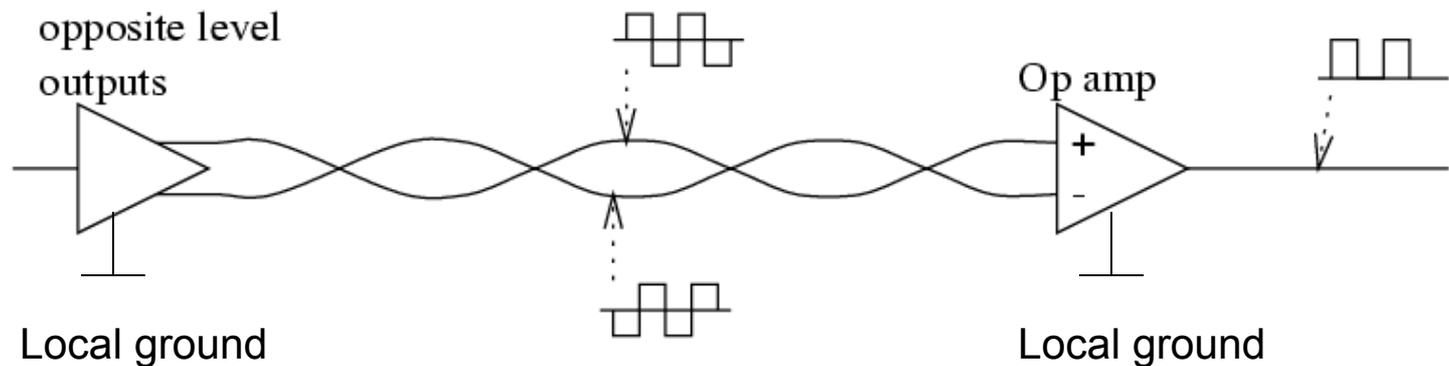
Combined with twisted pairs; Most noise added to both wires.
