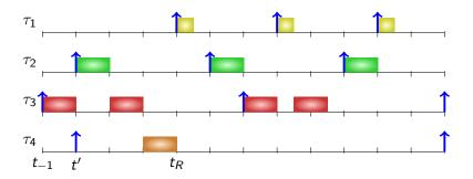
Shifting the release time of tasks together will increase the response time of task  $\tau_k$ .
