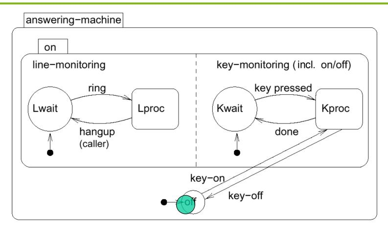
Line-monitoring and key-monitoring are entered and left, when service switch is operated.
