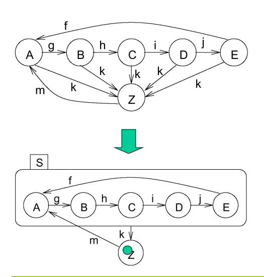
FSM will be **in** exactly one of the substates of S if S is **active** (either in A or in B or ..)
