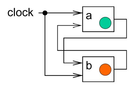
In an actual clocked (synchronous) hardware system, both registers would be swapped as well.
