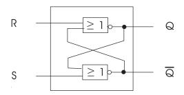
Describe this element's behavior in VHDL. Suppose that each NOR-gate gives rise to a delay of *1ns*. Declare all signals to be of type *Bit*. Draw the waveforms, given this component is stimulated as follows:
