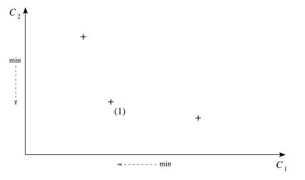
In the diagram, mark the area which is dominated by solution (1), i.e. mark all those alternative designs which are "worse" than design (1). Also, mark the area in which solutions would dominate design (1).
