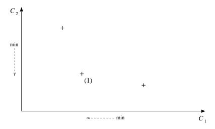
In the diagram, mark the area which is dominated by solution (1), i.e. mark all those alternative designs which are "worse" than design (1). Also, mark the area in which solutions would dominate design (1).
