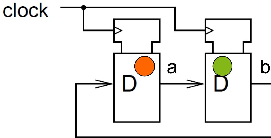
In an actual clocked (synchronous) hardware system, both registers would be swapped as well.
