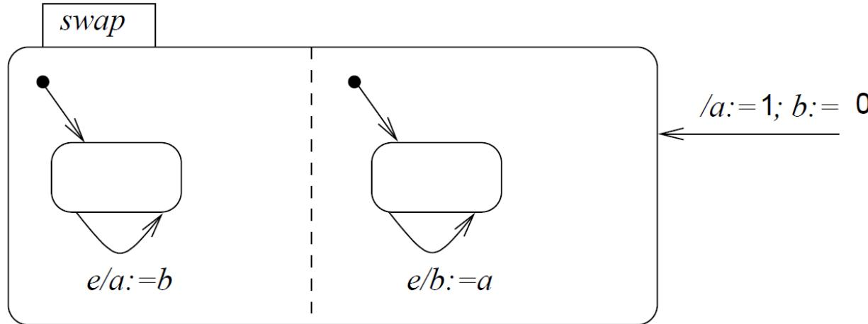
In a single phase environment, executing the left state first would assign the old value of  $b$  ( $=0$ ) to  $a$  and  $b$ :
